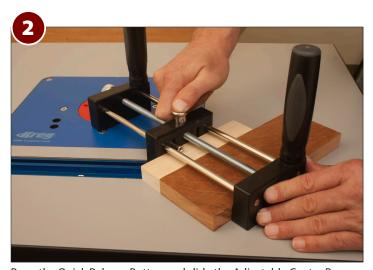
Press the Quick Release Button and slide the Adjustable Center Base over and against your stock piece while making sure that your stock piece is laying flat on your table top surface. Release the Quick Release Button. In this example we are using a sacrificial block to prevent tearout.
