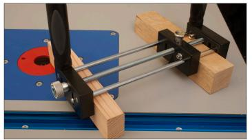
There will more than likely be times where you need to rout stock that is thicker than the Small Stock Holder. We recommend following these setup instructions. Create an "outrigger" by cutting a piece of stock that is the same thickness as your working stock piece. Attach the "outrigger" Stock piece to the Right Side Base of the Small Stock Holder through the slots using panhead screws (not included). Doing this will keep your Small Stock Holder and stock piece stable while routing.
