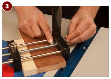
Using the Hex Key Wrench, loosen the Stock Hold Down Pins and slide them down until they are firmly against your stock piece. Secure each Stock Hold Down Pin with the hex key wrench. Next, using the Center Base Adjustment Knob, secure the stock piece by rotating the knob until the stock piece is firmly in place. Double check to be sure that your stock piece is still flat against your table top and is properly secured before proceeding to the next step.
