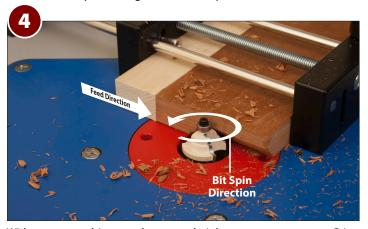
With your router bit set to the proper height, turn your router on. Grip the Small Stock Holder Handles and feed the stock into the router in the direction opposite of the router bits rotation. While feed your stock, be sure to keep the stock piece flat on the table and in contact with the router bit bearing guide
